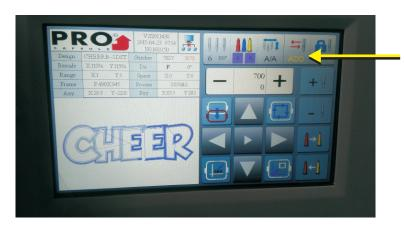
If you want to move forward by color, press the Embroidery Float button again until the on-screen icon displays **ADD**. You will now see 2 new buttons in the lower left corner of the display. The first one will move forward 1 color when pressed, and the second one will move back 1 color when pressed.
