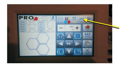
While the machine is embroidering it can move as many stitches you need backward just by pressing **STOP**. The machine will back up.
