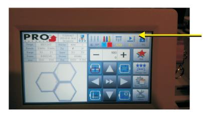
If you want to move forward quickly but not as fast as described above, press the Embroidery Float button again until the on-screen icon displays one arrow. When you press the **START** button the hoop will move forward through the design just as it does when the **STOP** button is pressed to move backward.
